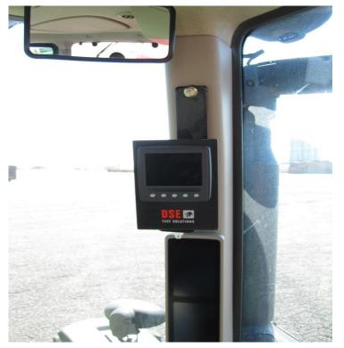
Avoid placing the Display in areas where it can be exposed to direct sunlight.
