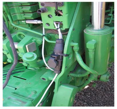
NB: These 7 pin trailer connectors are for DSE4200 use only and must not be connected to other equipment than DSE4200 or damage may occur.
